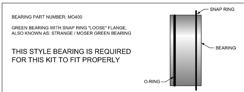
Figure 2. Loose Fit Bearing Configuration
